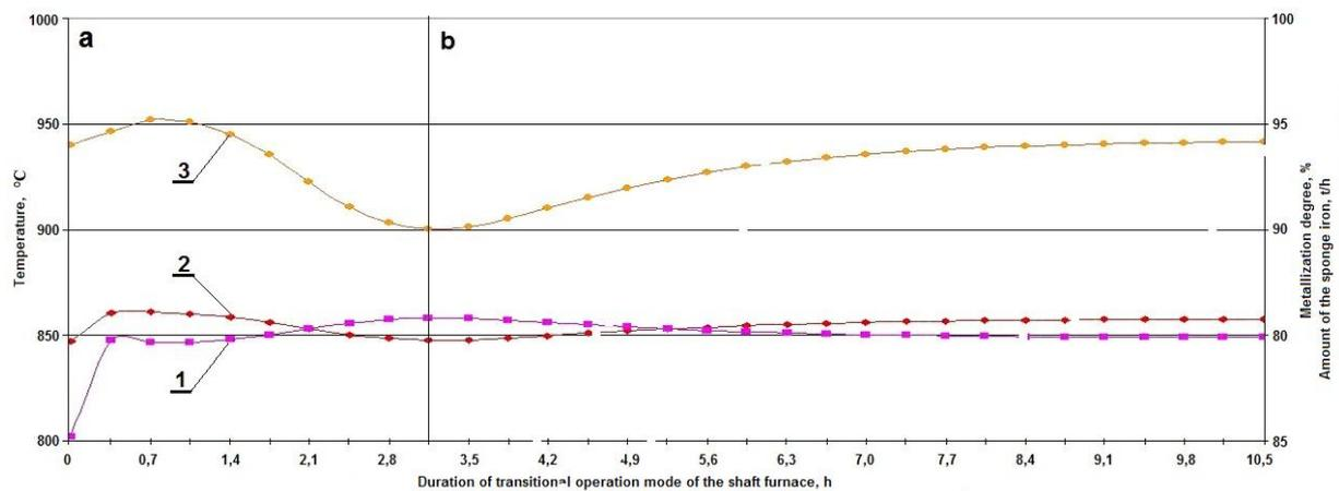
**Fig. 2** Dynamics of the sponge iron parameters at the output of the shaft furnace reduction zone (in the lower zone limit - 9,6 m from grate bar):
