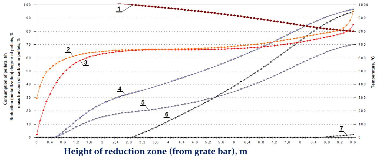
**Fig. 1** Distribution of the metallization process parameters within height of the shaft furnace.
